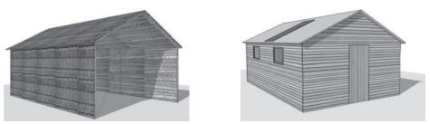
Semi-permanent house with wooden panels as wall and corrugated iron sheeting on the roof. The house is fitted with a solar panel for electricity.
