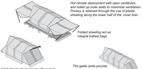
Cold climate deployment with sealed doors and vestibule to minimise ventilation and retain heat generated by stove The gable ends provide an overlapping seal when joining two or more modules end to end
