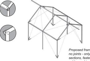
Proposed frame requires no joints - only equal angle sections, fasteners, tension cables and tensioners
